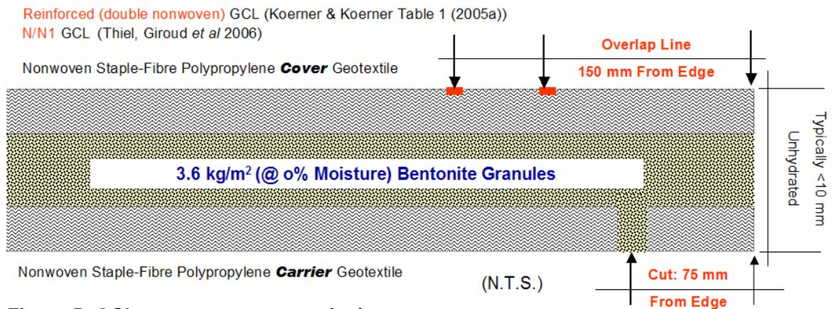
**Figure 5: GCL type nonwoven *carrier* / nonwoven *cover***
