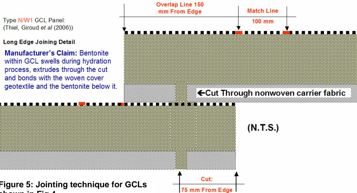
**Figure 5: Jointing technique for GCLs shown in Fig 4**
