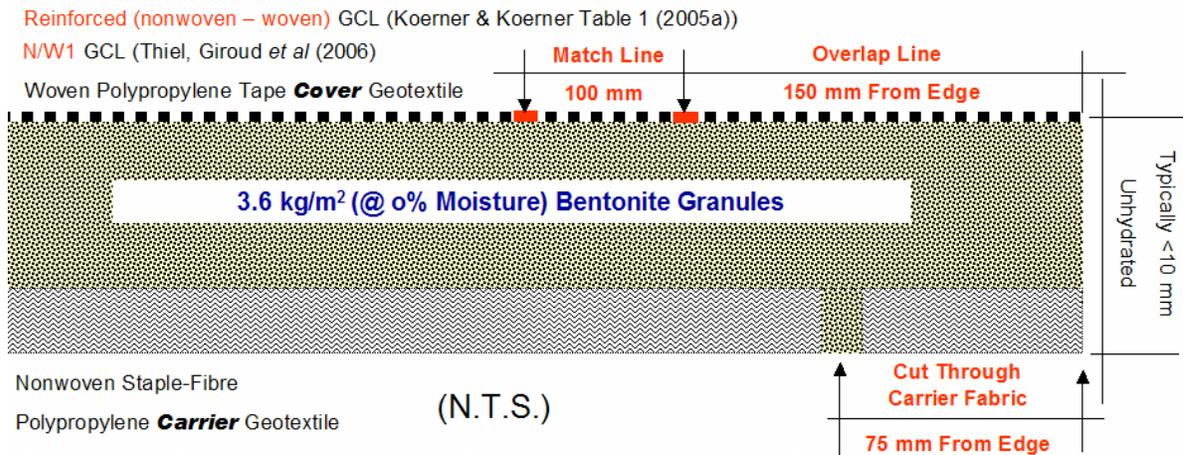
Figure 4: GCL type nonwoven carrier / woven cover
