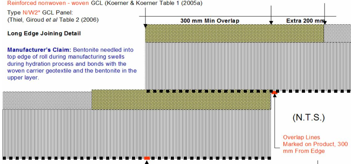
Figure 3: Jointing technique for GCLs shown in Fig 1 and Fig 2
