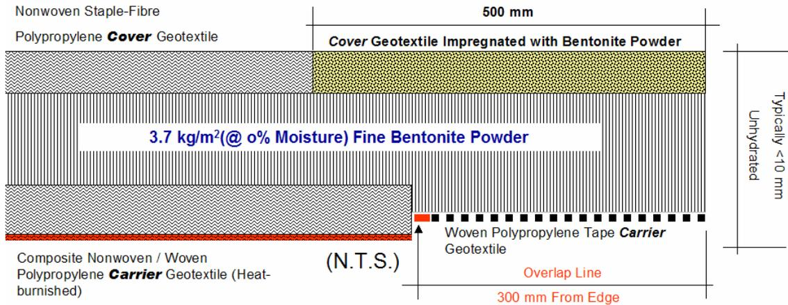
Figure 2: GCL type nonwoven cover / woven+nonwoven composite carrier
