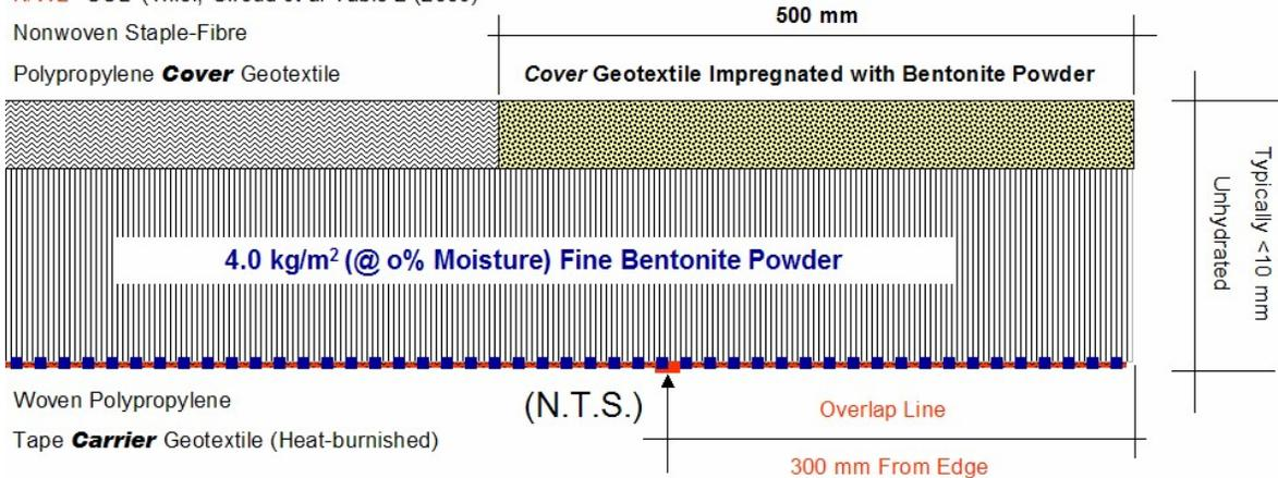
Figure 1: GCL type nonwoven cover / woven carrier
