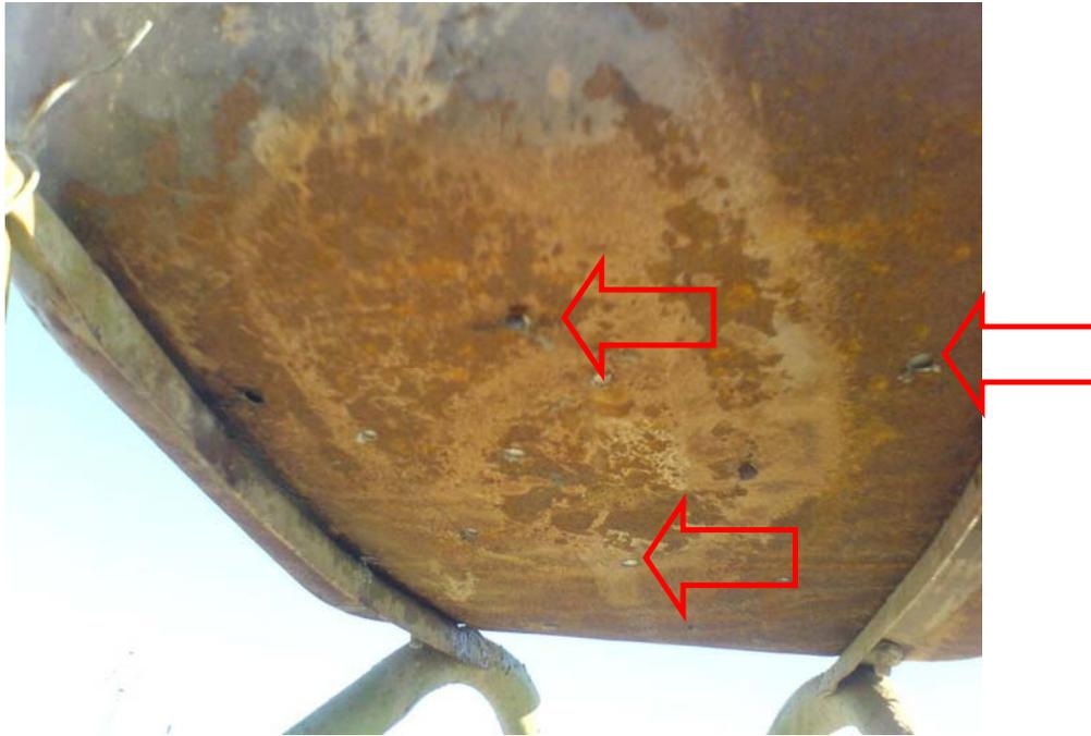
**Photo 3 : holes in the base of the wheelbarrow
