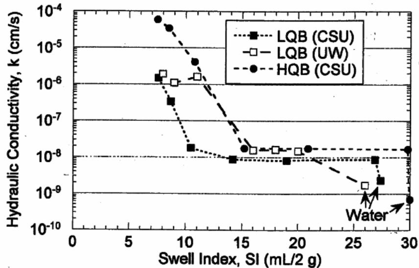
Figure 3. Hydraulic Conductivity of GCL as a function of free swell of bentonite from Lee et al (2005)
