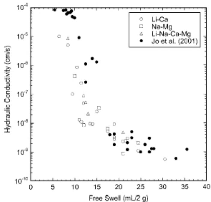
Figure 2. Hydraulic Conductivity of GCL as a function of free swell of bentonite from Kolstad et al (2004a)
