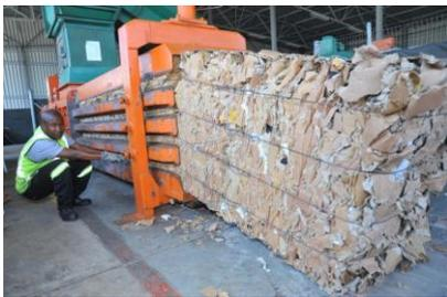
A worker at the baling machine in the GMSA Struandale Plants' recycling area which compacts and binds recyclable material before delivery to recyclers.
