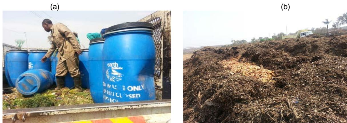
Figure 2. Delivery of Bokashi treated waste (a) and the addition of the waste to the windrows (b)
