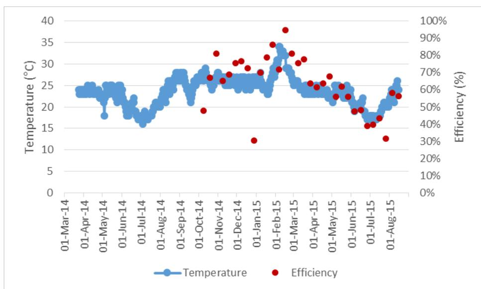
Figure 4. Temperature and efficiency in the Anaerobic Digester from March 2014 to August 2015
