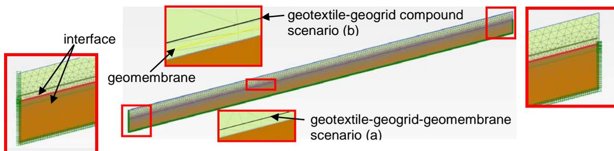
Figure 4. The schematic shape and the boundary conditions in numerical model
