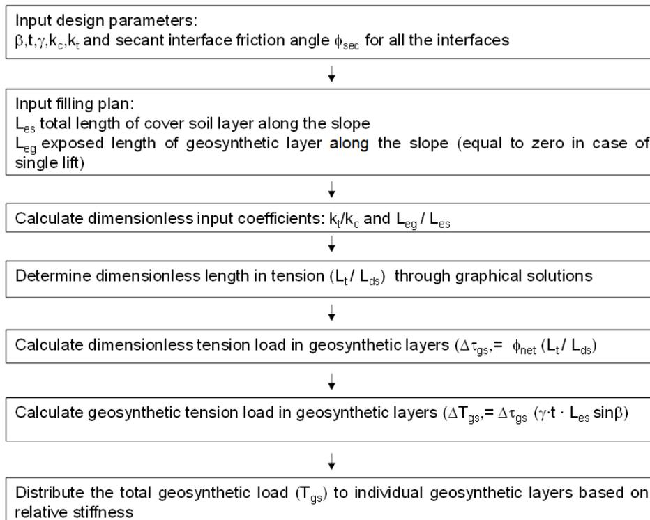
Figure 2. Procedure for estimating geosynthetic tension (modified from Liu and Gilbert 2005).
