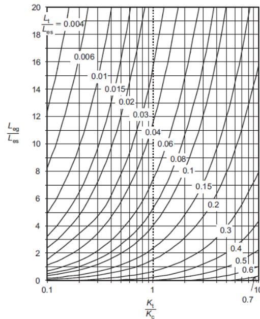
Figure 3. Graphical solution of Liu and Gilbert, (2005): length in tension,  $L_t/L_{es}$  against stiffness in ratio  $K_t/K_c$  and ratio of exposed length of geosynthetic layer to exposed length of placed cover soil layer,  $L_{eg}/L_{es}$  (adopted from Liu and Gilbert, 2005).
