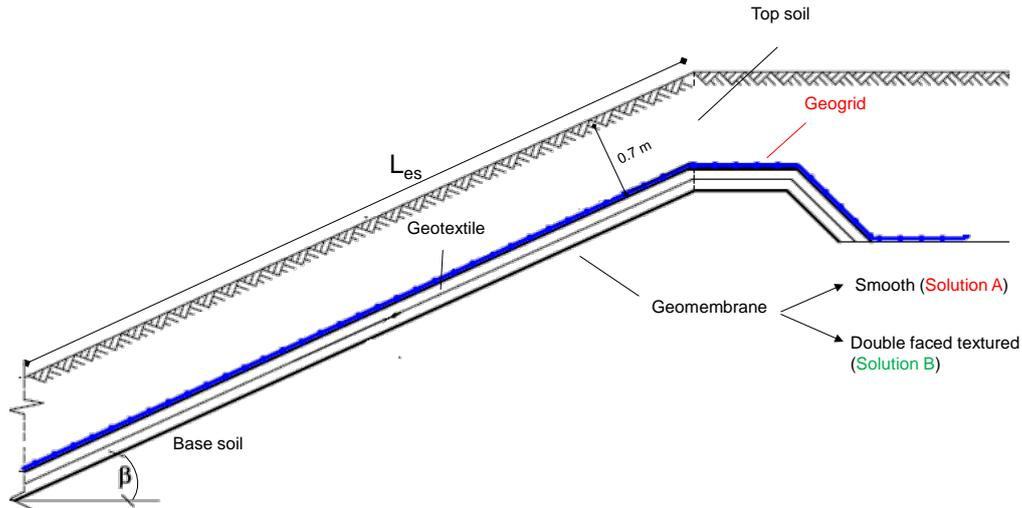
Figure 1. Scheme of the geocomposite liners considered in the study.
