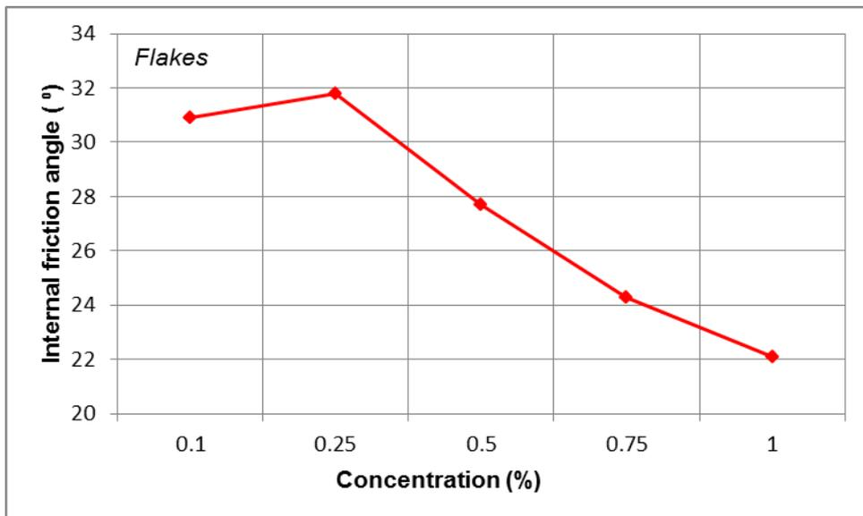
Figure 6b: Internal friction angle versus concentration (Flakes)
