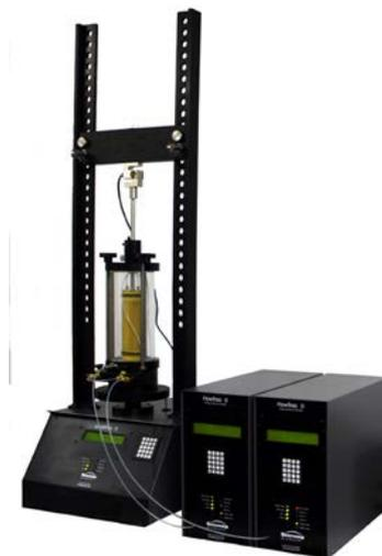
Figure 3. Geocomp LoadTrac-II/FlowTrac-II triaxial test system
