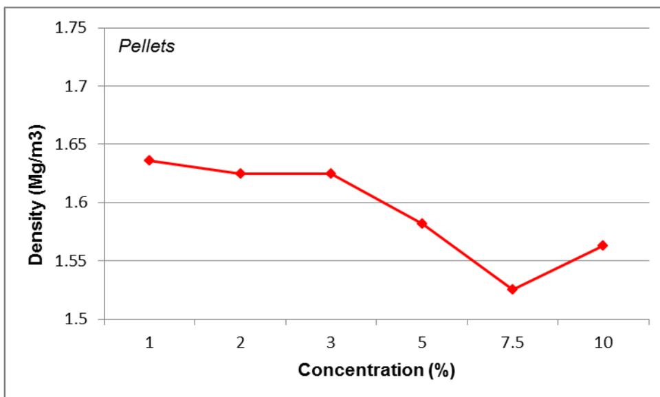
Figure 7a: Density angle versus concentration, pellets
