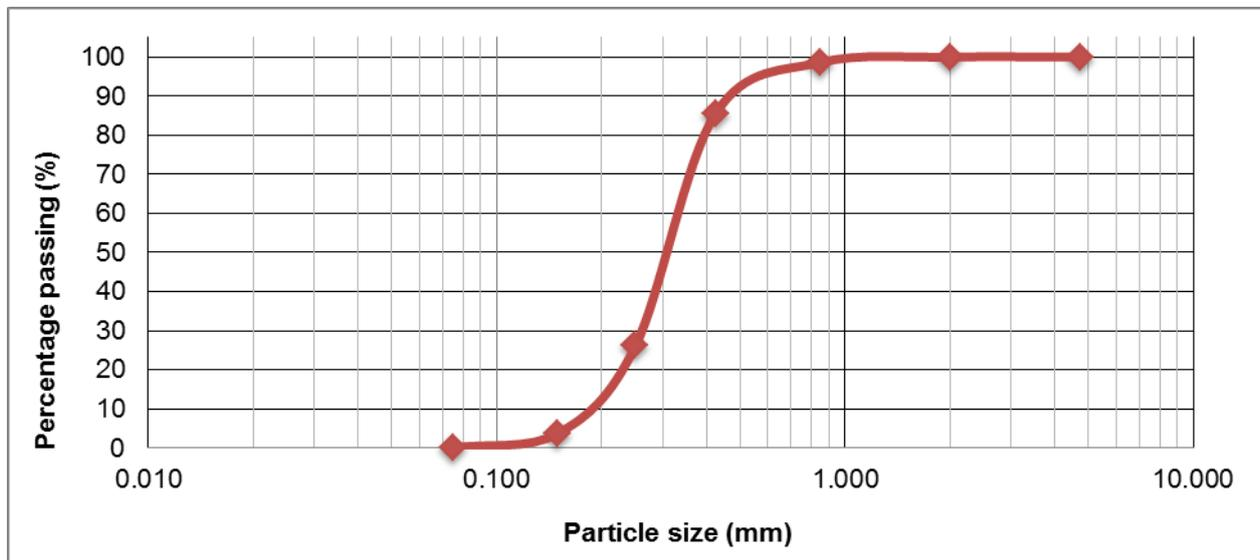
Figure 1. Particle grading curve
