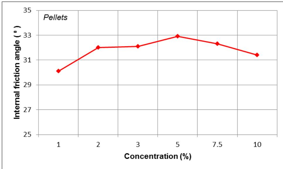
Figure 6a: Internal friction angle versus concentration (Pellets)
