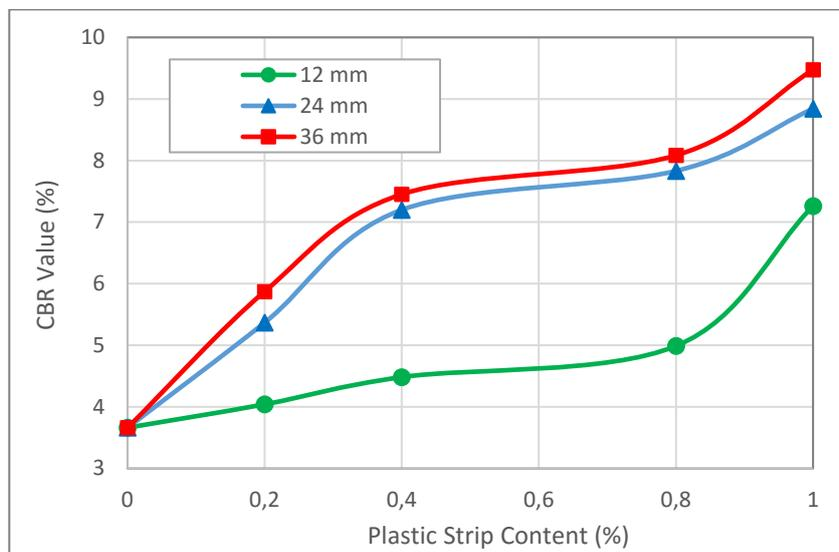
Figure 4. Graph of CBR vs Plastic Strip Content of Specimen
