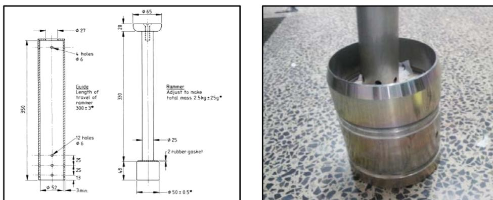
Figure 1. Compaction of soil-plastic composite specimen in the CBR mould
