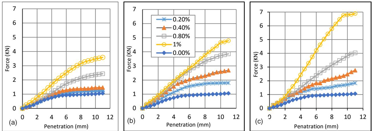
Figure 3. Graphs of Load vs Penetration for soil-plastic composite specimen with plastic strips of different aspect ratios and various plastic contents
