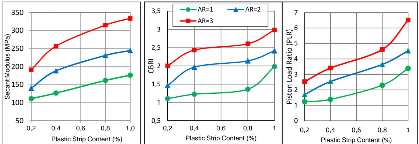
Figure 5. Graphs of different strength indexes vs plastic strip content at various aspect ratios
