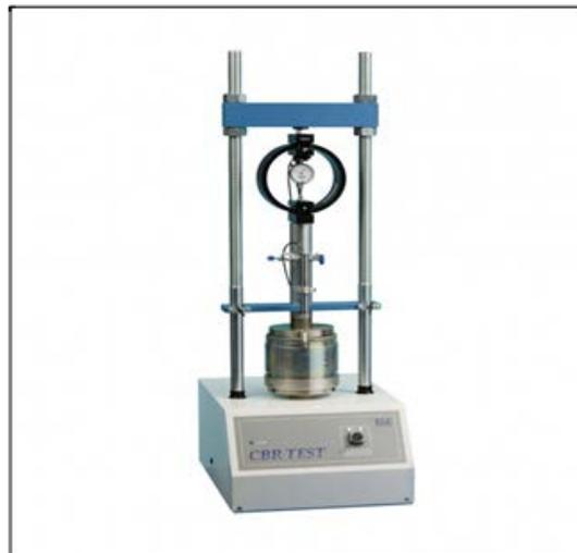
Figure 2. CBR Testing Equipment
