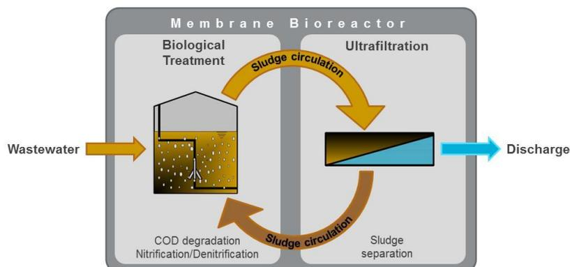
As the pore size of an ultrafiltration membrane lies around 0.02 - 0.05  $\mu\text{m}$ , no activated sludge is lost, i.e. biomass and suspended matter are retained in the biological system. The complete retention of biomass is a distinctive feature compared to conventional treatment systems and SBRs which two main beneficial effects: - the concentration of adapted bacteria can be kept at a high level - the partial-associated contaminants remain in the system, which improves effluent quality.
