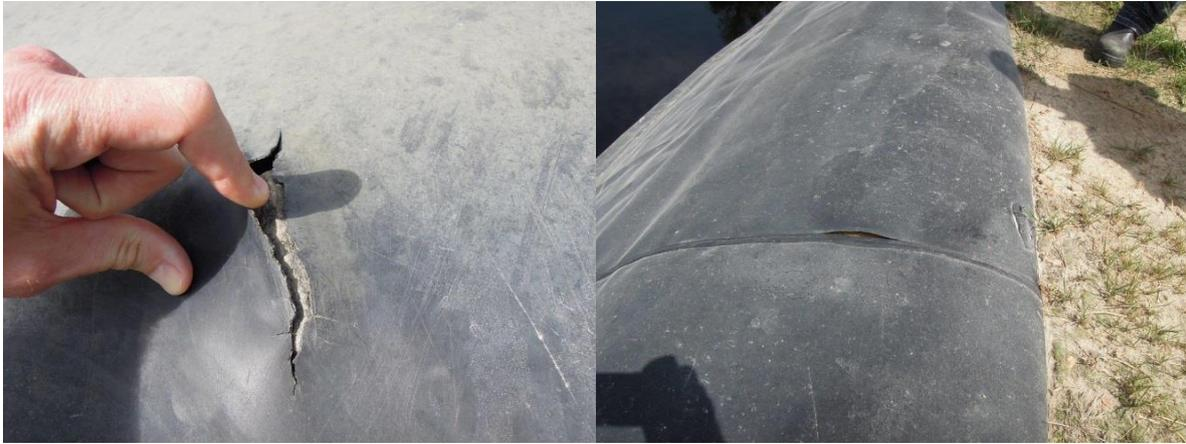
Figure 3. Stress cracking on exposed blown film fold in a stormwater dam.
