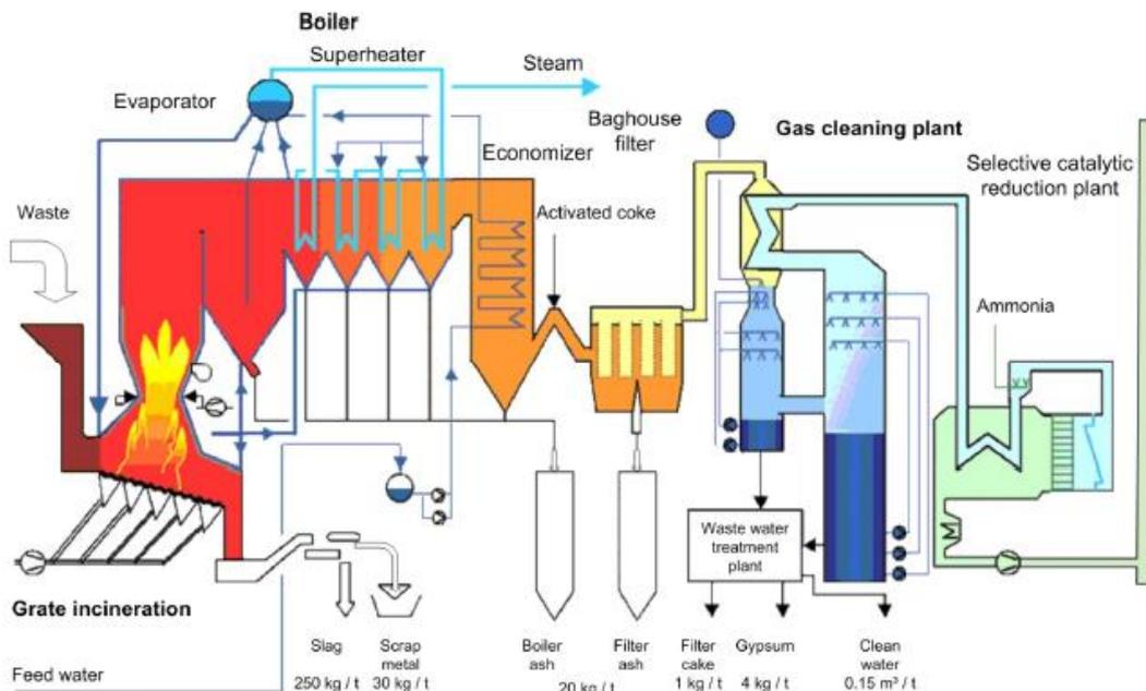
Figure 3: Grate Incineration plant with multistage flue gas treatment (UV&P, 2014)
