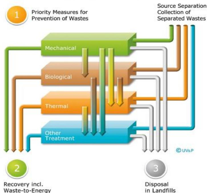
Figure 1: Typical Integrated system for sustainable waste management, UV&P, 2014.
