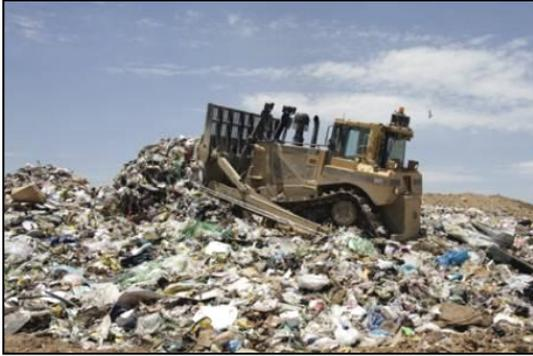
Figure 7: Track type tractor.
