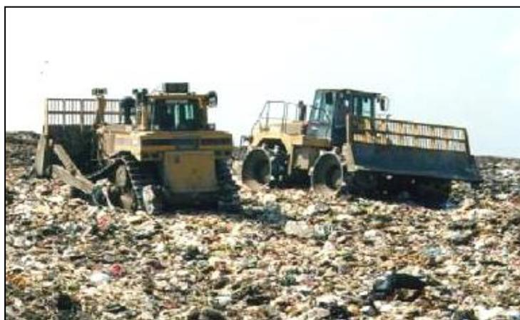
Figure 9. Left: Track type tractor spreading in thin layers. Right: Landfill compactor does straight passes
