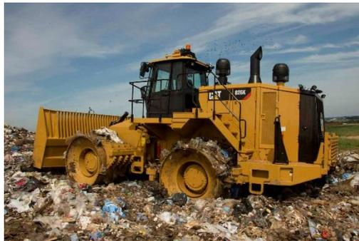
Figure 1: Landfill compactor in operation
