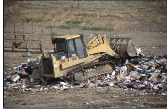
Figure 8: Track type loader
