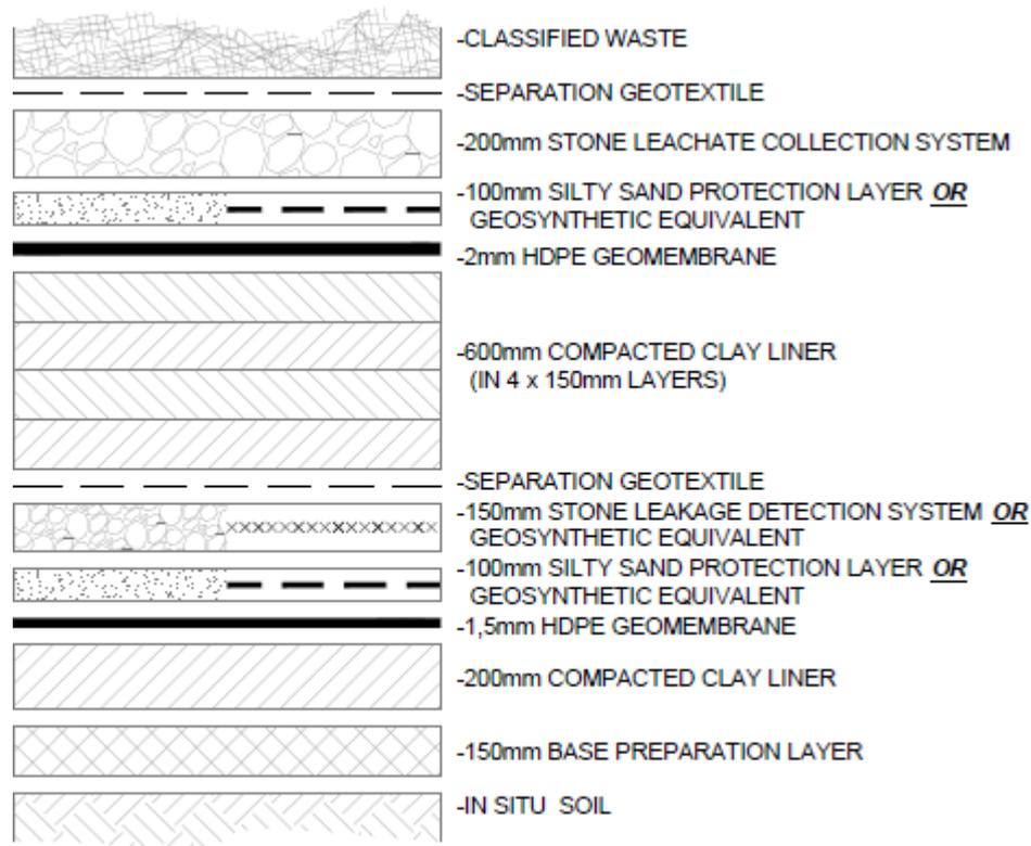
Figure 3. Class A Landfill Barrier (from the National Norms and Standards for Disposal of Waste to Landfill, Notice 636 of 2013).
