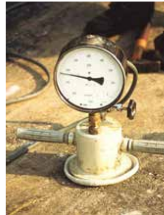
Figures 13 - Drill Cores Taken for Testing Impermeability and Vacuum Testing Joints
