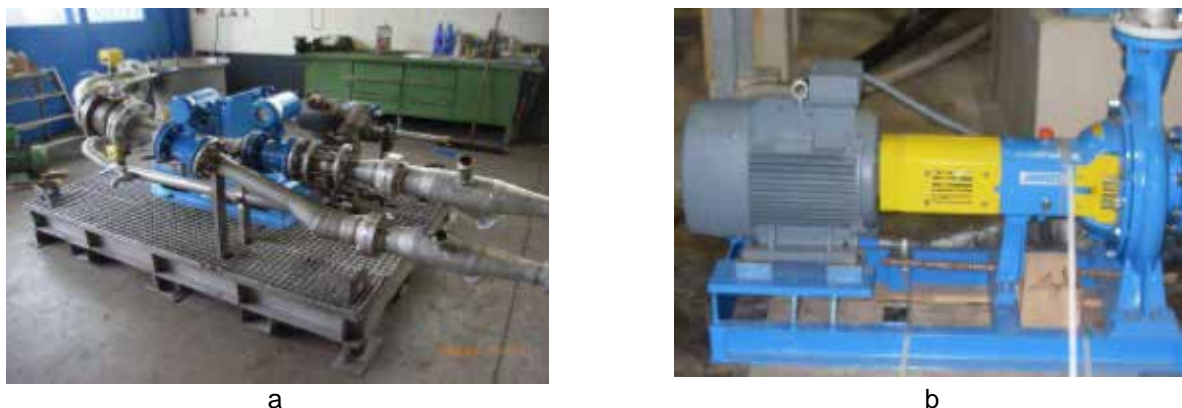
Figure 3: The two elements of the pressure screen: a) screen unit with installed pipes and measurement equipment and b) pump unit
