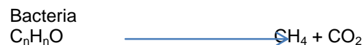
Figure 1: Simplified reaction of the methanogenesis where C n H n O represents the decomposable fraction of the waste.
