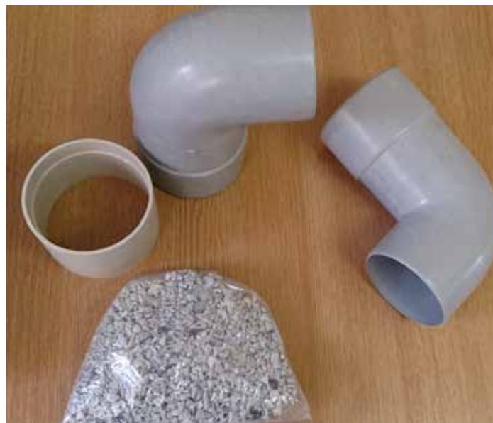
Figure 5: Guttering components manufactured from e-waste ABS plastics.
